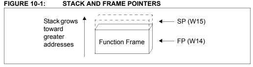
The C run-time startup modules in libpic30-omf.a initialize the Stack Pointer W15 to point to the bottom of the stack and initialize the Stack Pointer Limit register to point to the top of the stack. The stack grows up and if it should grow beyond the value in the Stack Pointer Limit register, then a stack error trap will be taken. The user may initialize the Stack Pointer Limit register to further restrict stack growth.
