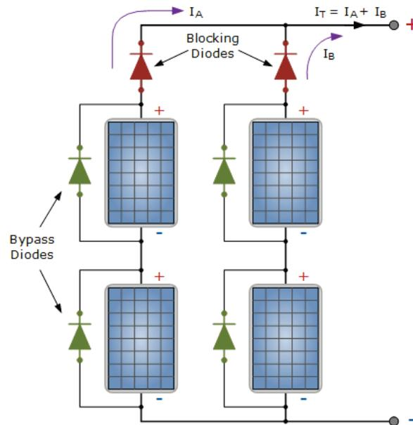
Figure 5. Example wiring diagram for solar cells in series and in parallel (taken from Sunbeam Systems<sup>30</sup>).
