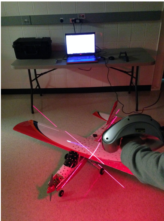
Figure 5: The Great Planes Avistar Elite being 3D scanned from above.
