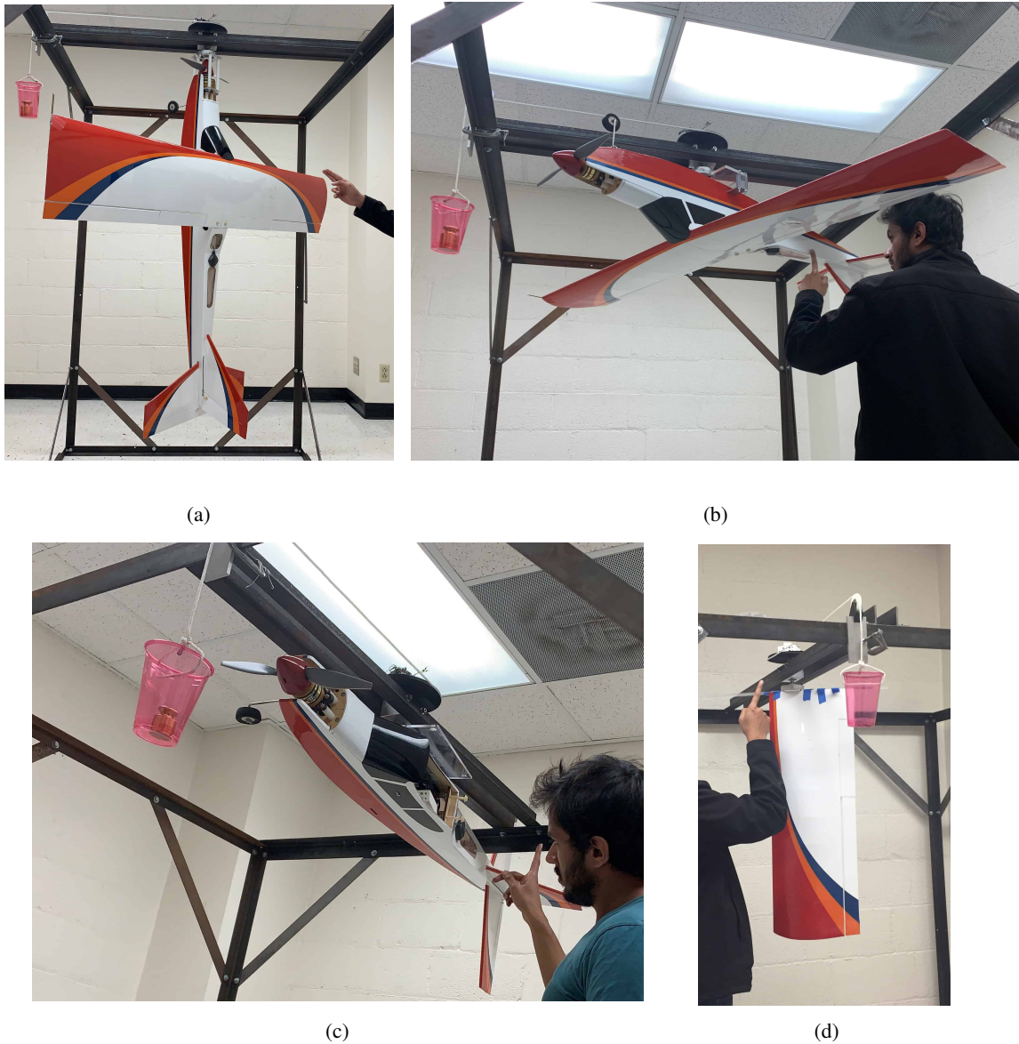
Figure 10: Moment of inertia testing of the flight-ready, instrumented Great Planes Avistar Elite about the (a) roll axis, (b) yaw axis, and (c-d) pitch axis.
