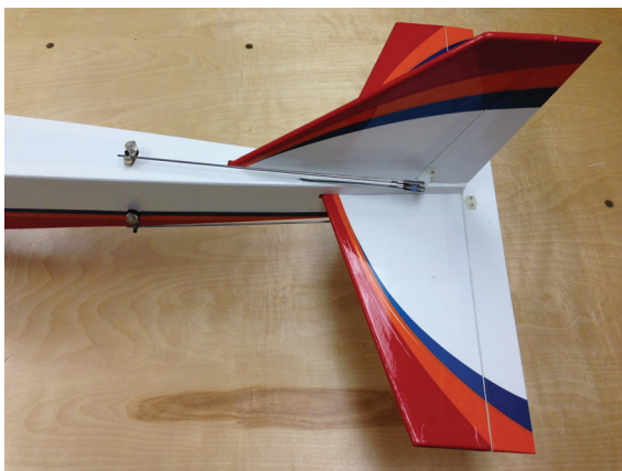
Figure 10. Elevator and rudder with potentiometers and linkages installed.
