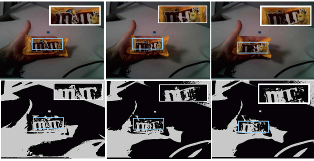
Figure 6. Tracked deformations of a candy wrapper (explanation in Fig. 4). The tracker correctly detects the increasing level of folding.
