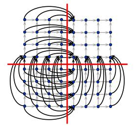
FIG. 4.3. A 2-TC-spanner of the grid with  $O(m^2)$  edges connecting vertices in different quarters. In addition to the depicted edges, it contains a transitive closure of each quarter and an edge from each vertex in the lower left quarter to the smallest vertex of the upper right quarter.
