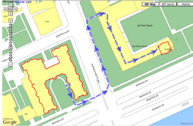
Figure 1: The user made the query shown at left; our method produced the result on the right. Our contribution is to compute efficient routes that seamlessly combine indoor and outdoor paths, allow different levels of granularity for source and destination, and cross 2D spaces not limited to the linear travel of automobiles.
