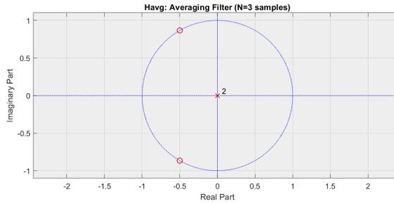
**Figure 3:** Pole zero plot of the Averaging Filter on the z-plane. The two conjugate zeros lie on the unit circle.
