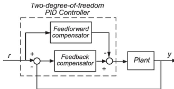
**Figure 8:** 2DoF PID Controller with feedforward(PD) and feedback(PID) compensator [1]
