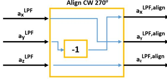
**Figure 16:** Accelerometer Alignment.
