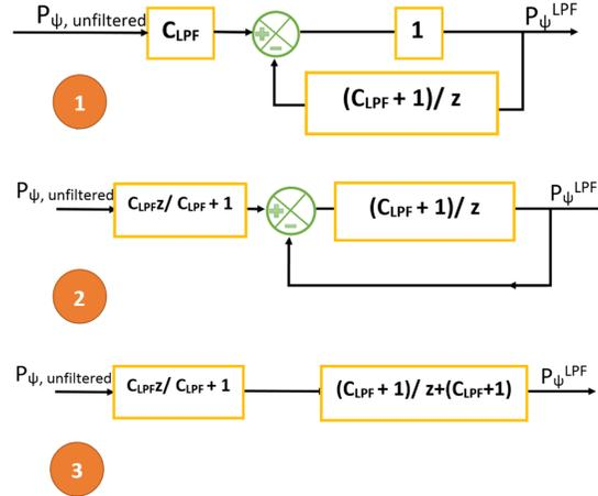
**Figure 9:** Block Diagram Representation of Proportional term's filter function for Yaw( $\psi$ ) axis. The graphical simplification steps are numbered in orange with step 1 depicting equation 45 and step 3 giving the final simplified form.
