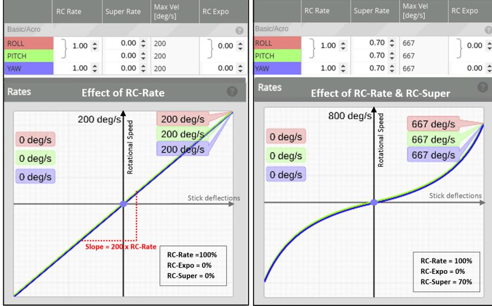
**Figure 5:** Left: Effect of RC Rates, Right: Combined effect of RC-Rates and RC-Super on the rotational speed v/s stick deflection curves for Roll, Pitch and Yaw channels. [3]
