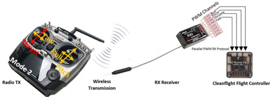
**Figure 2:** Transmitter-Receiver System with Parallel PWM communication protocol used between the four main receiver channels(roll: $\phi$ , pitch: $\theta$ , yaw: $\psi$  and throttle: $f$ ) and the Cleanflight flight controller running on top of an SPRACINGF3 board.
