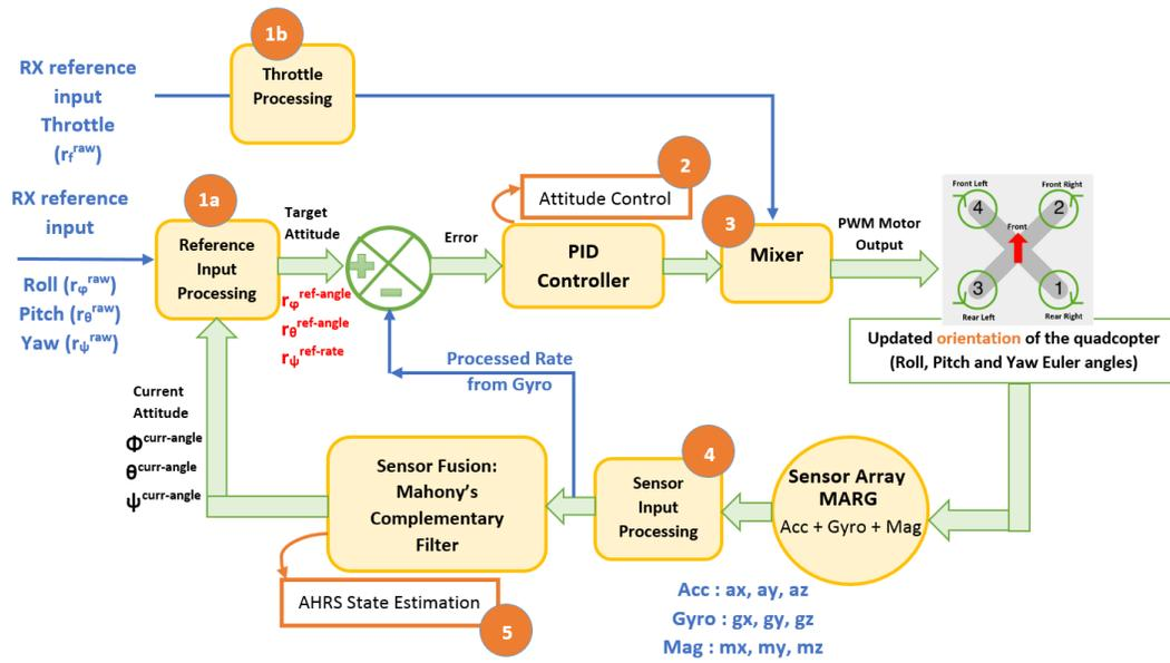
Figure 1: Cleanflight Flight/Attitude Control Loop
