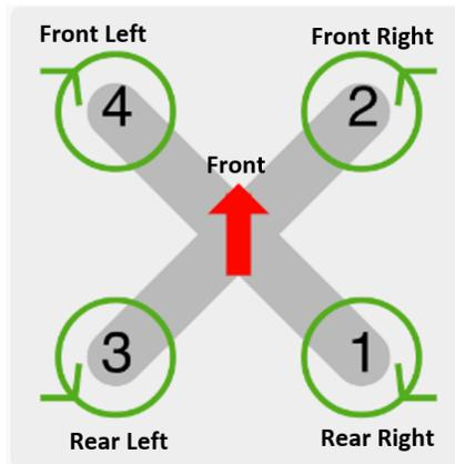
**Figure 13:** QuadX motor configuration and direction of rotation
