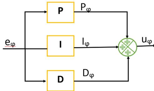
**Figure 7:** PID Controller for Roll Axis
