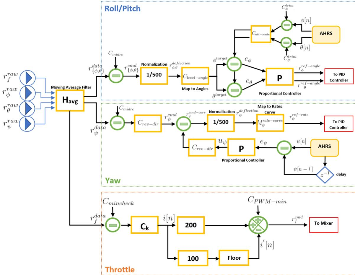
**Figure 6:** Processing of received data for Throttle, Roll, Pitch and Yaw user commands
