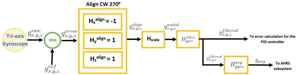
**Figure 21:** Gyroscope Data Processing with sub-component transfer functions presented as gains in yellow blocks.
