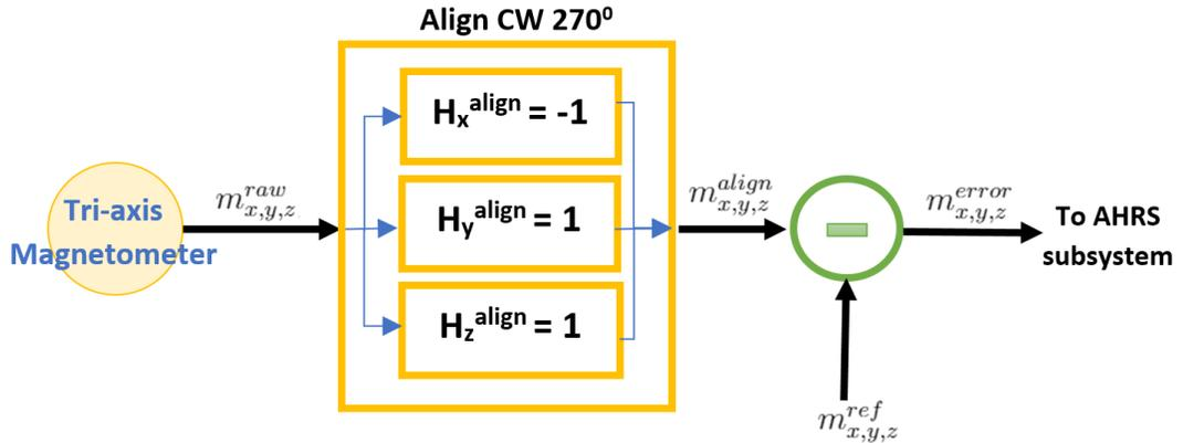
**Figure 19:** Magnetometer Data Processing.
