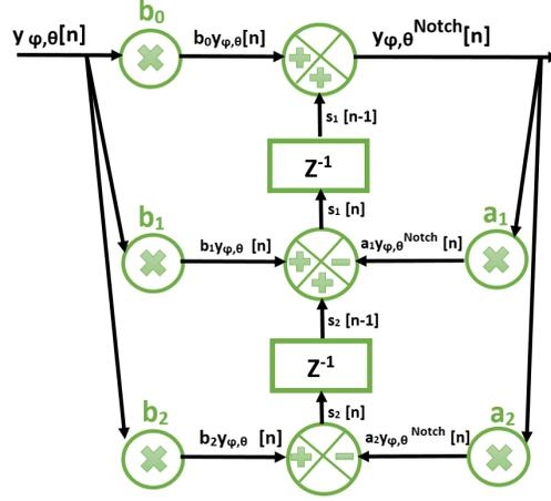
**Figure 12:** PID D term Biquad Notch filter for gyroscope data in direct form II topology
