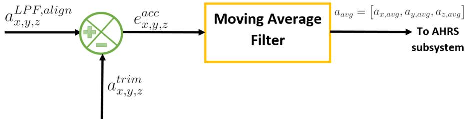
**Figure 17:** Accelerometer trimming and smoothing filter.
