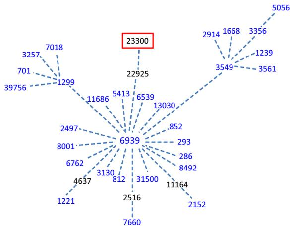
Figure 9: BGPPlay snapshot of prefix 64.72.205.0/24 (origin AS: 23300) which occurs in the smaller cluster.
