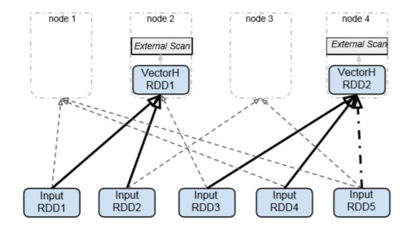
Figure 6: Mapping Spark RDDs to VectorH RDDs and ExternalScan operators Evaluation
