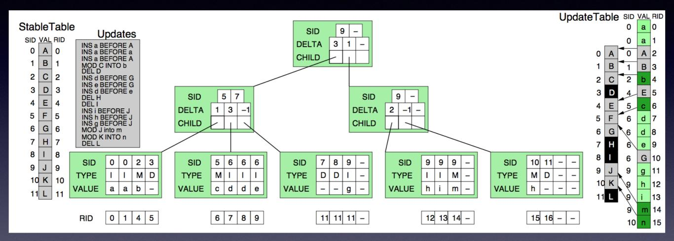
Merging in differences from a PDT is fast because it identifies tuples by position, rather than by primary key
