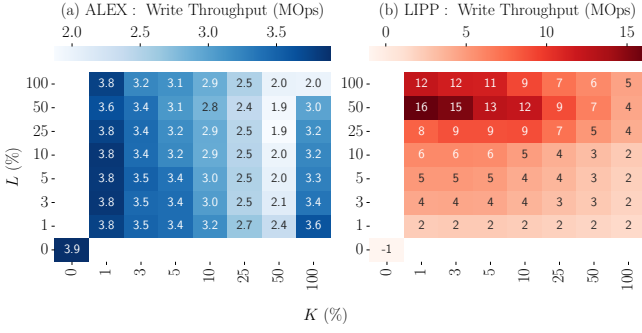
Figure 6: Ingestion Performance of learned indexes in stable-state: (a) ALEX offers better throughput when ingesting data with high sortedness; (b) LIPP performs better when the displacement of unordered entries ( L ) is larger for a fixed K .
