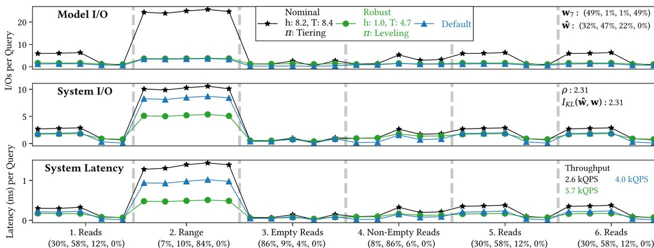
**Fig. 12** System and model performance for robust and nominal tunings in a read-only observed query sequence. Both tunings expected a mixed read-write workload. The tuning parameter  $\rho$  (input uncertainty)
