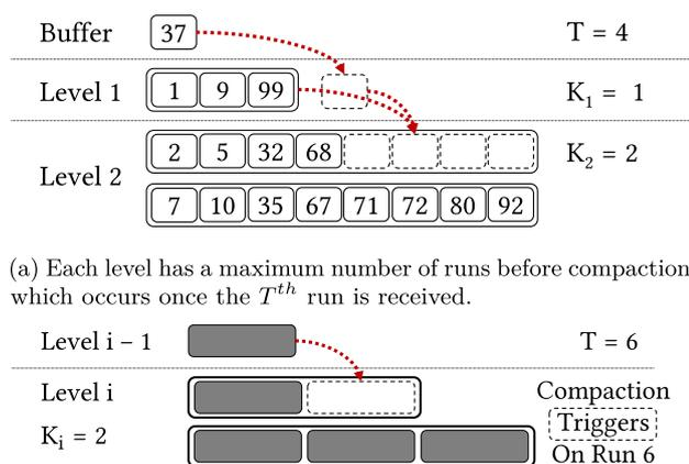
**Fig. 2** K-LSM provides a flexible way to describe different compaction behaviors. In this figure, assume the buffer is the same size as a logical page; then each sorted run is composed of multiple pages
