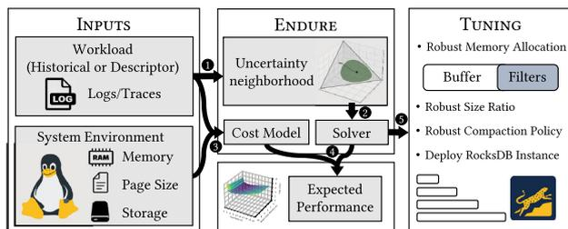
**Fig. 11** (1) Workload information is provided to ENDURE, establishing an uncertainty neighborhood centered on the expected workload. (2) This description of workload uncertainty is integrated into the solver. (3) The cost model receives both the workload and system parameter details. (4) Using the robust tuning from the solver and the cost model, an expected performance profile is generated. (5) The robust tuning is then deployed onto RocksDB
