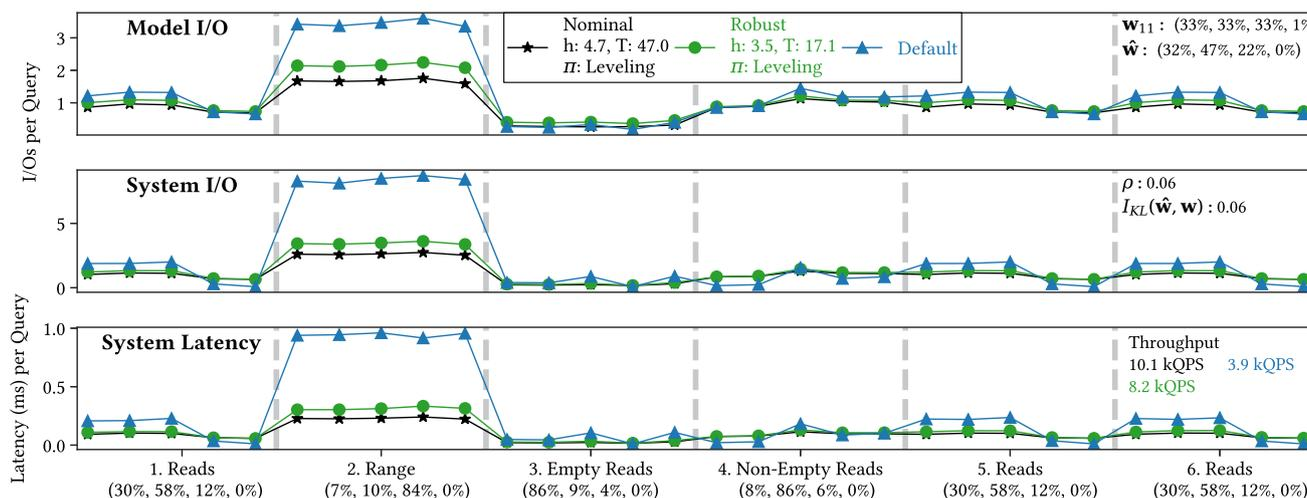
**Fig. 13** Read-only sequence where the observed workloads  $\hat{\mathbf{w}}$  is close to the expected, hence  $\rho$  and  $I_{KL}(\hat{\mathbf{w}}, \mathbf{w}_{11})$  deviate. Both tunings expected a read-heavy workload
