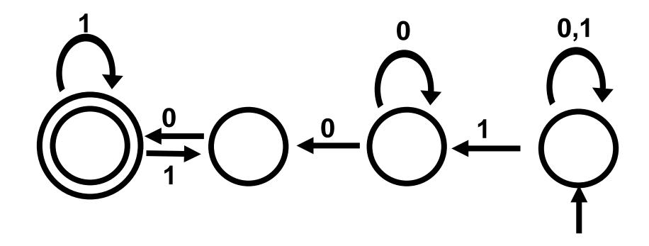
A Nondeterministic Finite Automaton (NFA) accepts if there exists a way to make it reach an accept state.
