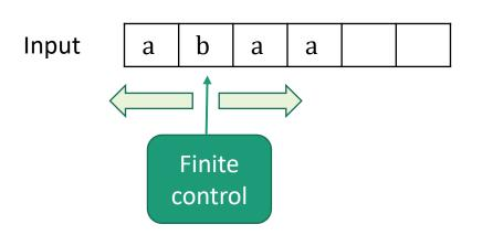
Control can scan in both directions Control can both read and write
