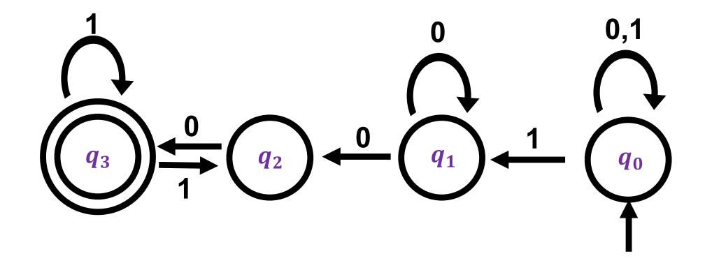
A Nondeterministic Finite Automaton (NFA) accepts if there exists a way to make it reach an accept state.
