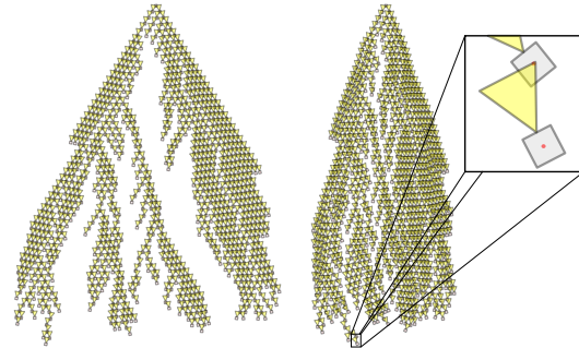
Fig. 7: A linear programming solution for a flock of 1024 robots which must maintain sensor contact squeezing together to fit through a doorway or hallway.
