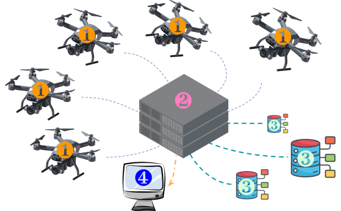
Fig. 2. A drone swarm, (1), sends data to a Data Processor server (2), which, in tandem, utilizes databases managed by Data Owners (3) to output the result to the Data User (4)
