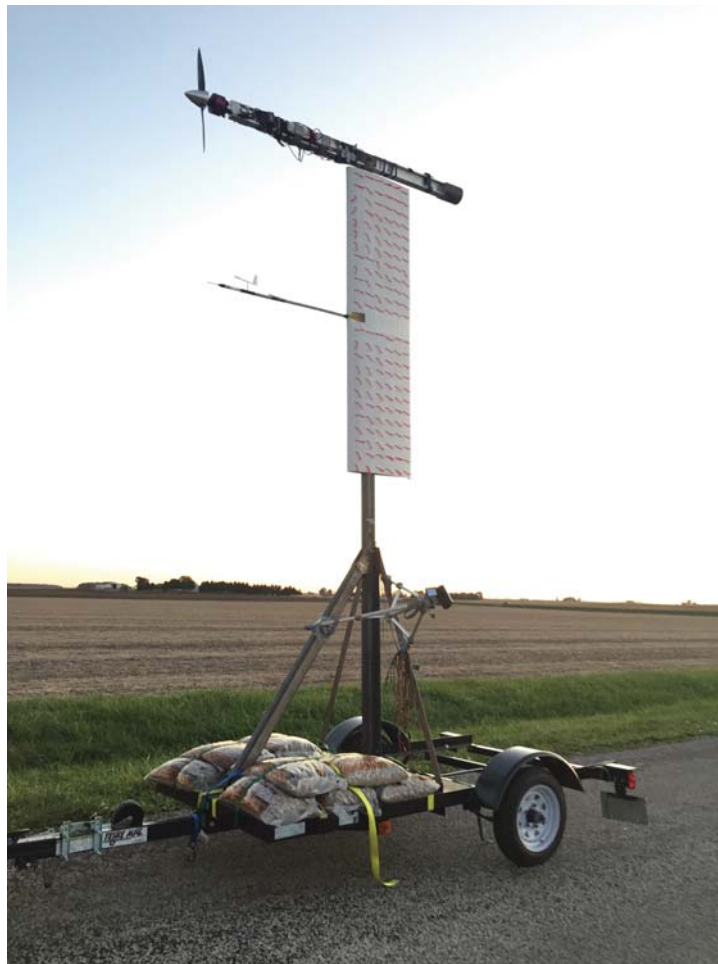
Figure 7. Tufts placed on the vertical beam fairing of the rolling rig to visualize airflow.
