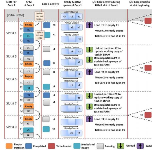
Fig. 3. Interaction between I/O Core and Core 1 for task scheduling.
