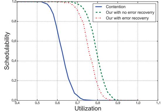
Fig. 9. Schedulability degradation when applying the recovery mechanism
