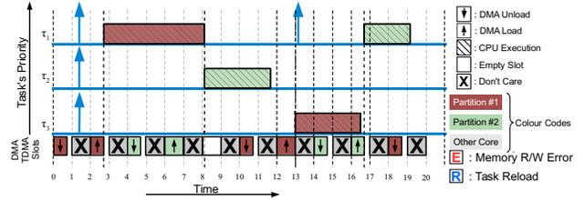
Fig. 4. Arbitrary scheduling example showing CPU, DMA and local memory
