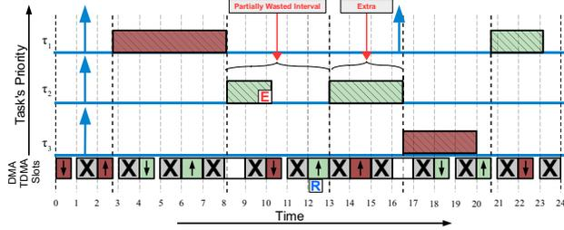
Fig. 5. The scheduling example with the proposed error recovery mechanism
