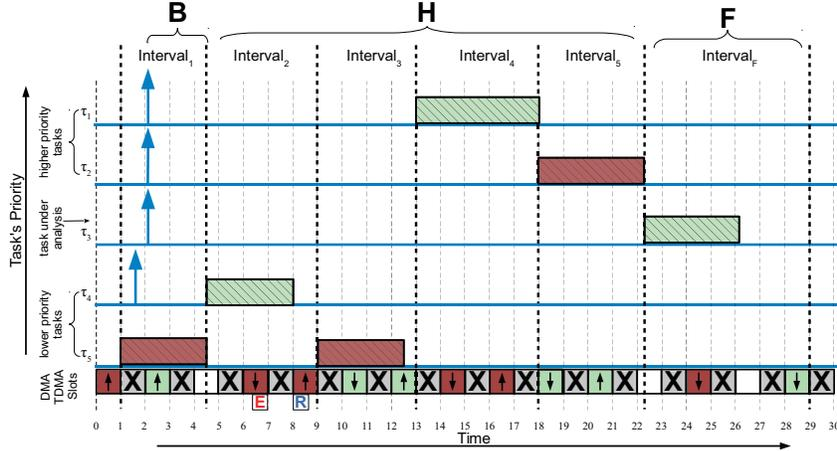
Fig. 7. Example showing how  $H$  is extended by an induced interval due to error recovery prior to  $Interval_F$
