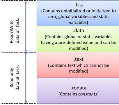
Fig. 2. Different sections of a task.
