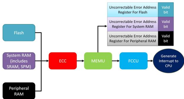
Fig. 8. Block diagram of error handling circuitry.
