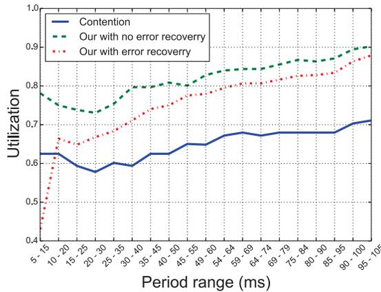
Fig. 10. Utilization degradation as a function of tasks periods
