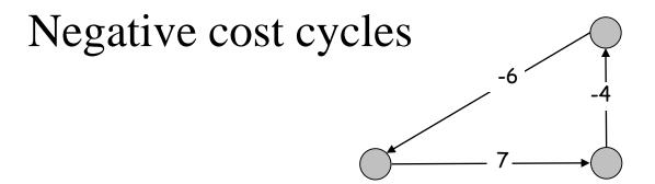
Observation. If some path from s to t contains a negative cost cycle, there does not exist a shortest s-t path; otherwise, there exists one that is simple.
